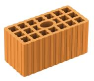
**Brick n.2** Category c: Hollow masonry: **Doppio UNI (12.12.25)** Bulk density class ρ=0.9 kg/dm<sup>3</sup> Minimum compressive strength fb=6.0 MPa
